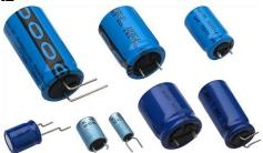
For our radial products we can offer special lead styles (J-, L-, Z-, V-, T-lead). The J-lead for example can be used for inverse-polarity protection. Next to that we do offer 3-pin radials. The benefit of 3-pins is that you do not need any additional fixation and the parts can handle a higher vibration compared to conventional 2-pin solutions.
