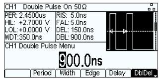
An additional modulation mode allows the delay between pulses to be modulated.
