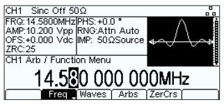
Standard waveforms include Sine, Rectangular, Ramps, Sin(x)/x, Haversine, Logarithmics, Exponentials, Gaussian/Lorentz and Cardiac.
