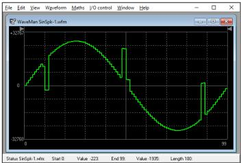
The program offers direct import from .csv files, the most commonly used format for graphical description. Additionally a Clipboard import function supports any waveform that can be described by a set of Y-axis data points regardless of their format.
