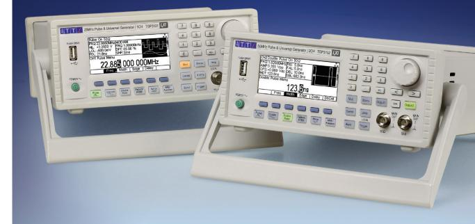
Advanced Pulse and Universal Generators - Single or Dual Channel True pulse generator operation including low jitter asynchronous pulses 50MHz pulses, 0.1ns period and delay resolution, fully variable rise/fall 50Mbps pulse pattern generation up to 65536 bits with preamble Noise generator with user-defined bandwidth and amplitude density High performance 50MHz/800MS/s arbitrary/function generator Programmable via USB, GPIB and LXI compliant LAN interfaces
