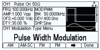
The modulation source can be internal or external. A very wide range of internal modulating waveforms are available.
