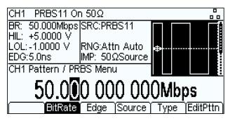
A PRBS is generated by a linear-feedback shift register with taps that generate a feedback signal via an exclusive-OR gate. The number of stages determines the sequence length (2N-1) whilst the clock frequency determines the bit rate.
