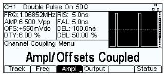
Outputs of the two channels can be coupled such that switching the output on/off on one channel switches the output on/off of both channels.
