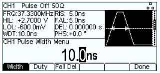
Pulse repetition frequency can be set between 1mHz and 50MHz (25MHz for TGP312x models) with up to 11 digits of resolution.
