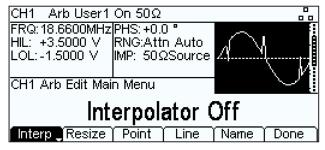
Waveform length is up to4096 samples. Four waveforms can be stored within the instrument with unlimited numbers available using the Flash drive interface or uploaded from the digital interfaces.
