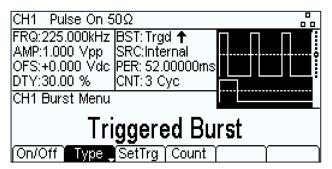
Triggered bursts can be from 1 to 4,294,967,295 cycles or infinite.
