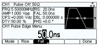
Rise and fall can be set together, or set independently. There are no limitations on rise time imposed by the pulse width.
